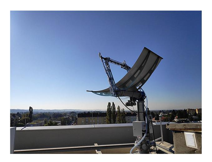
The parabolic trough collector is manufactured using industrial production methods such as injection molding. Credit: EMS-TU Graz
