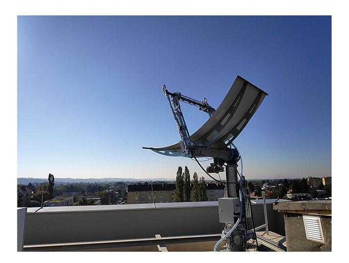
The parabolic trough collector is manufactured using industrial production methods such as injection molding. Credit: EMS–TU Graz
