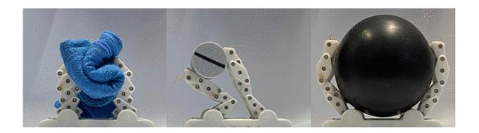
The gripper switches between three modes, which are suited to tasks that require maintaining a secure hold on an object or applying high pressure, precise finger positioning or in-hand manipulation, and passive adaptation to the shape of larger, delicate, or irregularly shaped objects. Credit: Harvard SEAS
