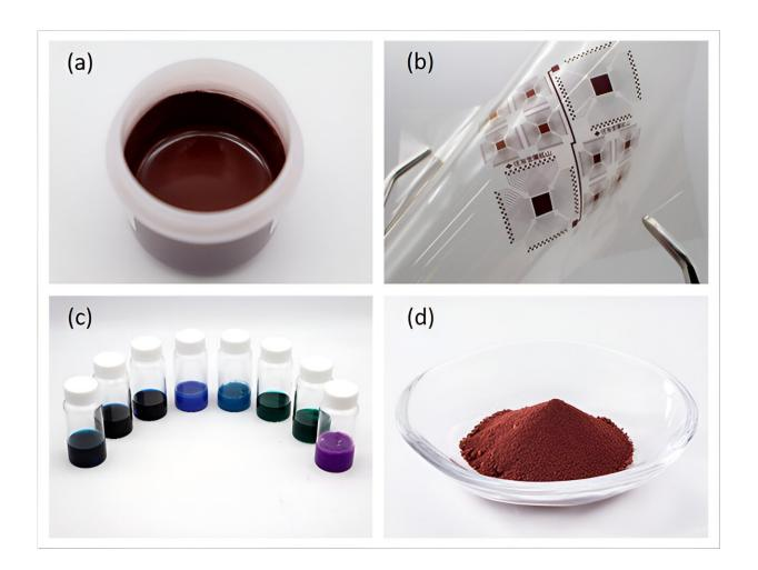
(a) Thick-film conductive ink. (b) Flexible substrate with patterns printed on its surface using the thick-film conductive ink. (c) Variety of metal complex inks that are used to synthesize the thick-film conductive ink. (d) Copper particles. Credit: National Institute for Materials Science
