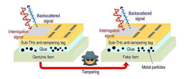
After passing through the tag and striking the object's surface, terahertz waves are reflected, or backscattered, to a receiver for authentication. Credit: Ruonan Han, Eunseok Lee, et al
