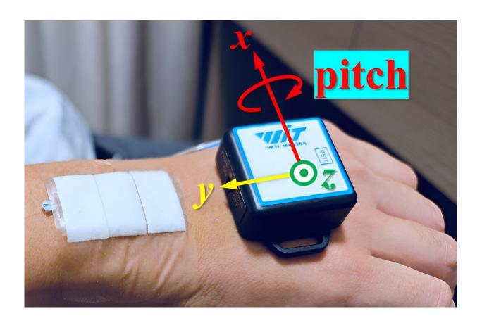
Researchers have developed a wearable PDMS sensor that uses a FBG to sense movements. The sensors could be used to monitor wrist, finger or even facial movements. Credit: Kun Xiao, Beijing Normal University in China
