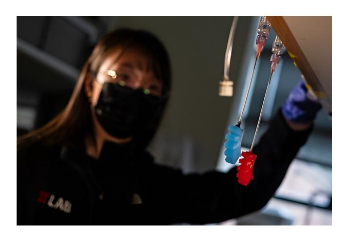
Te Faye Yap, a Rice University Ph.D. student in the Preston lab and lead author on a study published in *Cell Reports Physical Science*, demonstrates the performance of grippers cured at room temperature (blue) and at elevated temperatures (red) when pressurized. Credit: Jeff Fitlow/Rice University
