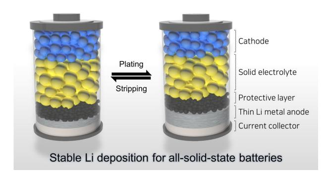
Diagram depicting the stabilization of a lithium metal anode-based all-solid-state battery through the bottom electrodeposition mechanism. Credit: POSTECH
