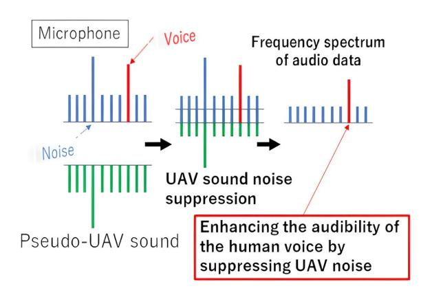
The innovative AI-based noise cancelling method generates a similar sound as the UAV noise and then substracts that sound from the sound captured by the UAV microphone to eliminate noise and therefore amplify human sounds. Credit: Chinthaka Premachandra/Shibaura Institute of Technology
