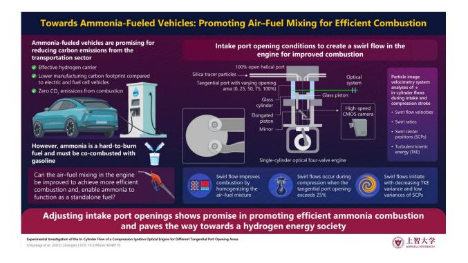
Swirling flows, initiated when the tangential port opening exceeds 25%, have the potential to enhance the mixing of air and fuel. This can result in a more homogeneous mixture, leading to improved combustion efficiency and reduced emissions. Credit: Mitsuhisa Ichiyanagi/Sophia University
