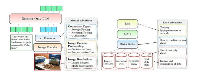
Left: Model ablations: what visual encoder to use, how to feed rich visual data, and how to connect the visual representation to the LLM. Right: Data ablations: type of data, and their mixture. Credit: *arXiv* (2024). DOI: 10.48550/arxiv.2403.09611
