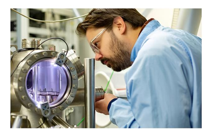
Dr Taylor Stock loading a sample into the scanning tunnelling microscope (STM), used to perform atomic scale fabrication. Credit: Agnese Abrusci/UCL
