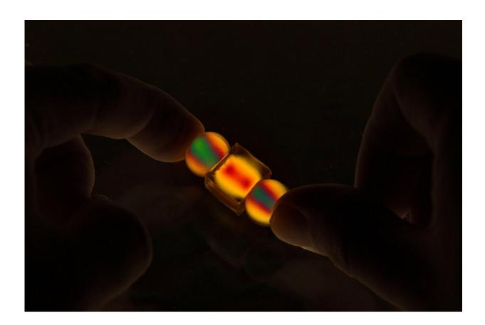
MIT researchers developed a method that allows for 3D experiments that can reveal how forces are transmitted through granular materials, and how the shapes of the grains can dramatically change the outcomes. In this photo, 3D photoelastic particles light up and change color under external loads. Credit: Ruben Juanes
