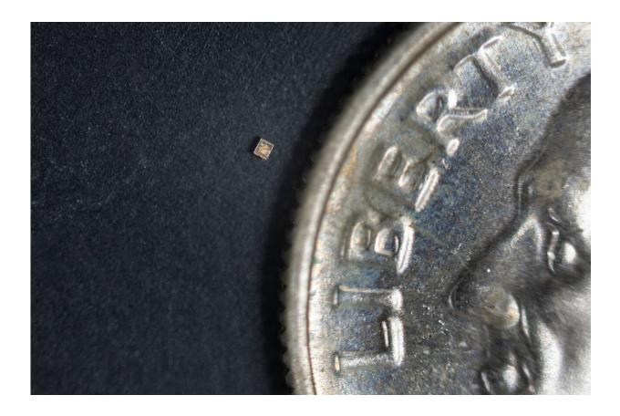
The sensor network is designed so the chips can be implanted into the body or integrated into wearable devices. Each submillimeter-sized silicon sensor mimics how neurons in the brain communicate through spikes of electrical activity. Credit: Nick Dentamaro/Brown University
