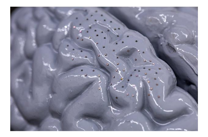
Writing in *Nature Electronics*, the research team describes a novel approach for a wireless communication network that can efficiently transmit, receive and decode data from thousands of microelectronic chips that are each no larger than a grain of salt. Credit: Nick Dentamaro/Brown University
