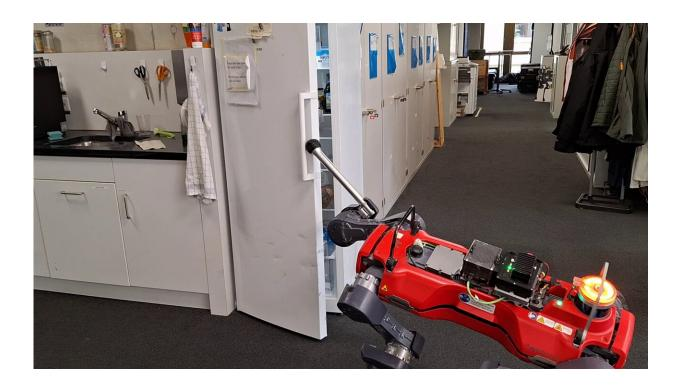
The legged robot ANYmal opens a fridge door using pedipulation. Credit: ETH Zurich.
