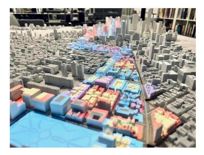
An interactive model demonstrates how a computer simulation framework, developed by Frank Li at Rensselaer Polytechnic Institute, can be used for city planning. Credit: Fengqi Li/ORNL, U.S. Dept. of Energy
