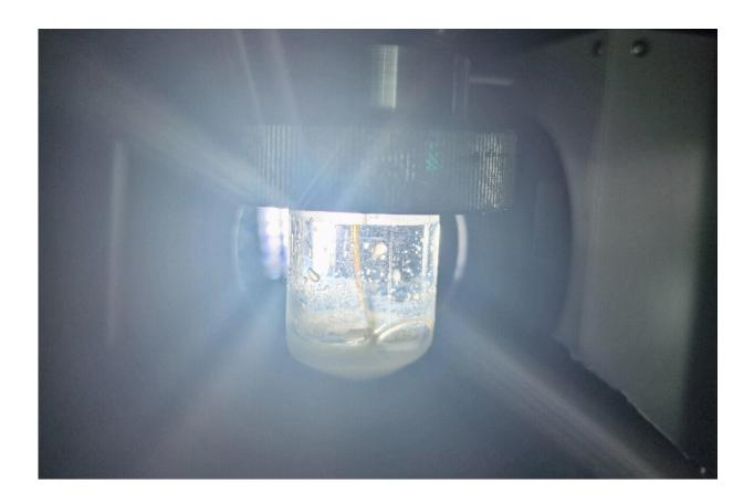
Reactor where the catalyst is tested for turning  $CO_2$  to methanol. Credit: University of Nottingham
