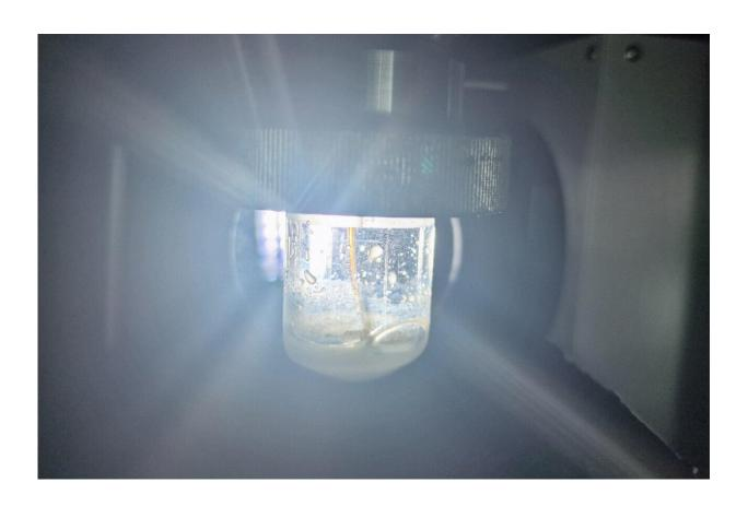
Reactor where the catalyst is tested for turning CO<sub>2</sub> to methanol. Credit: University of Nottingham
