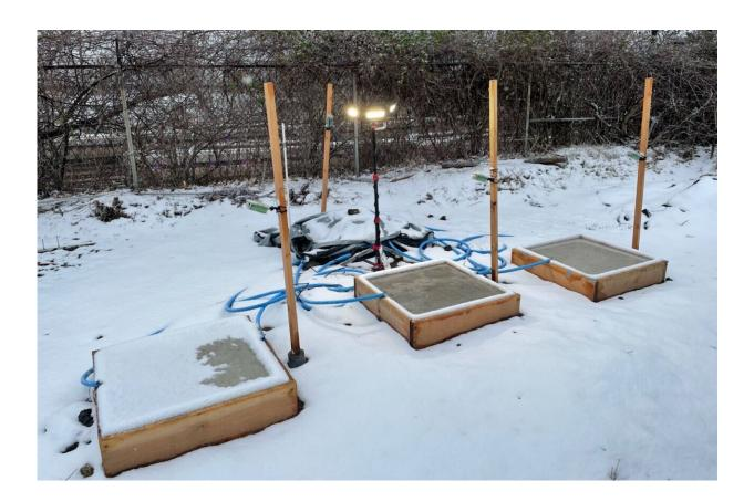
Drexel University researchers have tested concrete slabs containing phasechange material that can warm themselves up when temperatures fall in order to melt off snow and ice. [Left to right: reference slab, slab containing lightweight aggregate treated with phase-change material; slab containing microencapsulated phase-change material]. Credit: Drexel University
