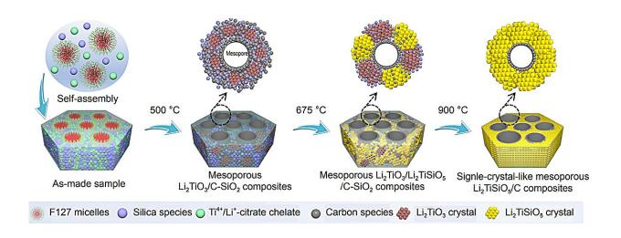
The strategy for the construction of the single-crystal-like mesoporous  $Li_2TiSiO_5$  is illustrated. The stoichiometric  $Ti^{4+}/Li^+$ -citrate chelate (SCP) was prepared as the precursor for the micelles directed self-assembly. Subsequent step-crystallization process leads to the formation of single-crystal-like mesoporous  $Li_2TiSiO_5$ . Credit: Science China Press
