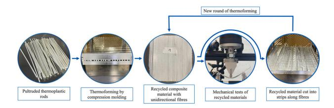
Basic layout of the study: glass fiber-reinforced polypropylene rods are heated and pressed into plates, which are then repeatedly cut into strips and pressed into plates again. The effects of such recycling on material properties are monitored. Credit: Valentina Kravtsova et al./Composites Communications
