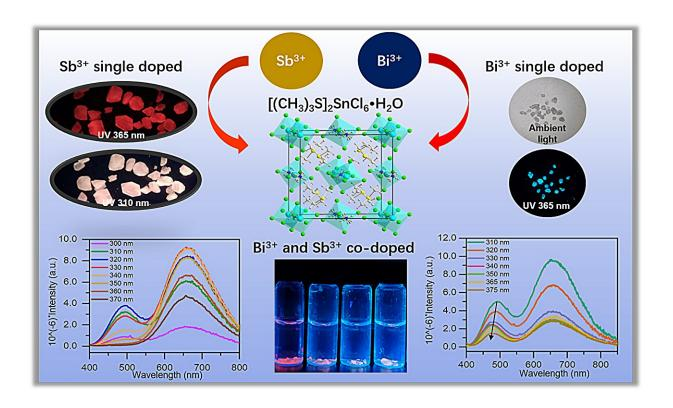
Luminescence properties of Sb<sup>3+</sup> doped andBi<sup>3+</sup>/Sb<sup>3+</sup> co-doped [(CH<sub>3</sub>)<sub>3</sub>S]<sub>2</sub>SnCl<sub>6</sub>×H<sub>2</sub>O. Credit: Yitong Lin, Yu Zhong, Yangpeng Lin, Jiawei Lin, Lei Pang, Zhilong Zhang, Yi Zhao, Xiao-Ying Huang, Ke-Zhao Du
