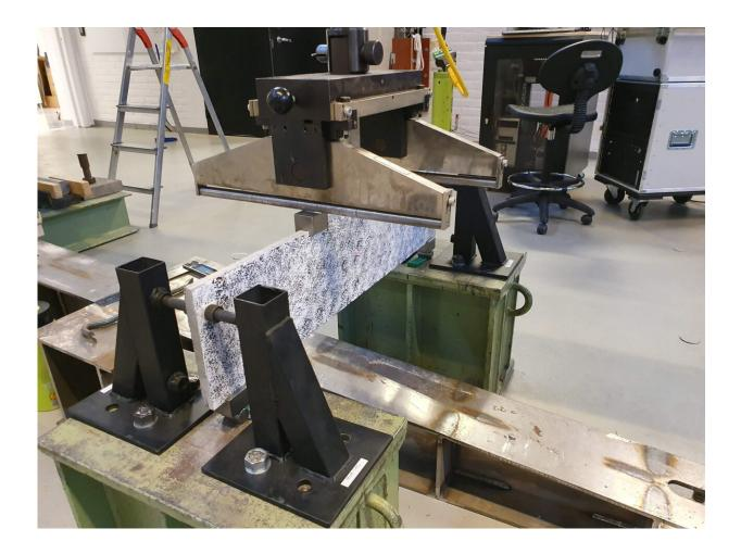
Test set-up where textile-reinforced concrete is loaded in the Structures Lab at Chalmers. Credit: Chalmers University of Technology | Sebastian Almfeldt
