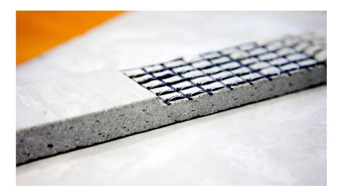
Concrete reinforced with carbon fiber textile. Credit: Stipriaan | Wikimedia Commons
