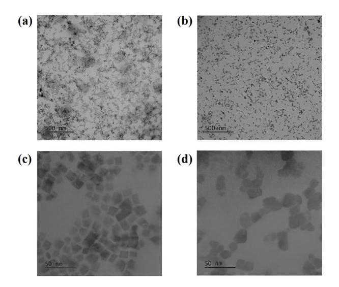
TEM images of (a and c) pristine-PQD and (b and d) IPA-treated PQD with different magnifications. Credit: *Advanced Energy Materials* (2024). DOI: 10.1002/aenm.202304276
