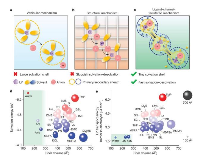
Electrolyte design and solvent-screening strategies.  $\mathbf{a}-\mathbf{c}$ , Schematic illustrations of Li<sup>+</sup> transport behaviors with the vehicular mechanism ( $\mathbf{a}$ ), structural mechanism ( $\mathbf{b}$ ) and ligand-channel-facilitated mechanism ( $\mathbf{c}$ ).  $\mathbf{d}$ , The solvation
