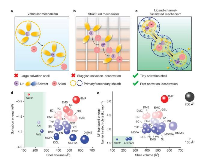
Electrolyte design and solvent-screening strategies. **a–c**, Schematic illustrations of Li<sup>+</sup> transport behaviors with the vehicular mechanism (**a**), structural mechanism (**b**) and ligand-channel-facilitated mechanism (**c**). **d**, The solvation
