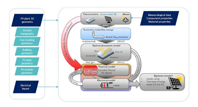
Flow of the physics-based energy yield simulation framework. Credit: IMEC
