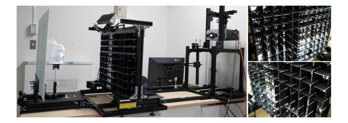
The entire configuration of the system (left): from left to right, the projection target, mirror-lens array, projector for projection mapping, and projector for illumination. A close-up of the mirror-lens array. This configuration reflects rays emerging from the lens array, leading to an increased ray density (right). Credit: Assocaite Professor Yoshihiro Watanabe
