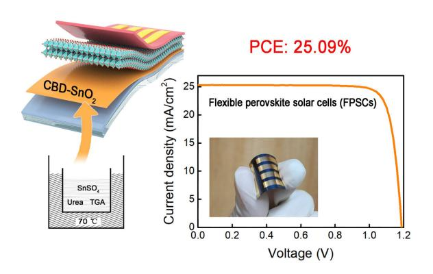
$SnSO_4$  is used as a tin precursor for the tin oxide ( $SnO_2$ ) deposited as the electron transport layer of FPSCs. A new CBD manufacturing method allows more control over  $SnO_2$  growth, improving the overall power conversion efficiency of the solar cell and increasing the practicality of flexible solar cell technology. Credit: iEnergy, Tsinghua University Press
