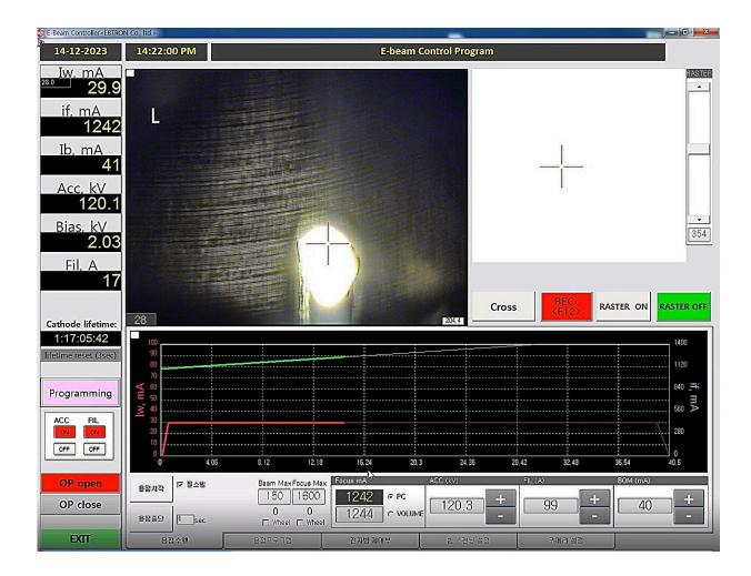
Welding operation screen using the electron beam welder. Credit: Korea Electrotechnology Research Institute(KERI)
