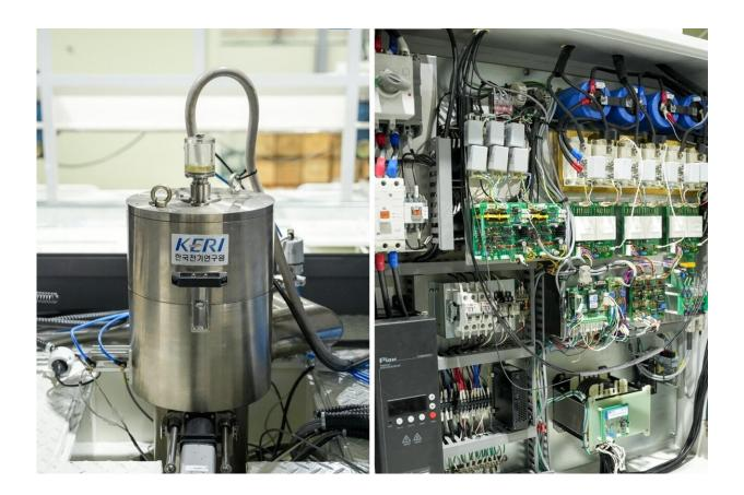
Electron beam welder's 'electron guns' (left) and 'parts of power supplies' (right). Credit: Korea Electrotechnology Research Institute (KERI)
