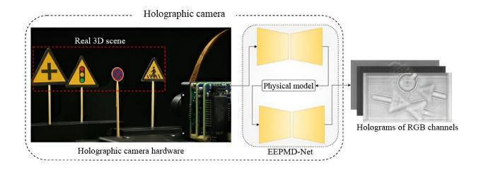
The proposed holographic camera mainly consists of a liquid camera based on a large-aperture liquid lens and an end-to-end physical model-driven network. Credit: Di Wang, Zhao-Song Li, Yi Zheng, You-Ran Zhao, Chao Liu, Jin-Bo Xu, Yi-Wei Zheng, Qian Huang, Chen-Liang Chang, Da-Wei Zhang, Song-Lin Zhuang, and Qiong-Hua Wang
