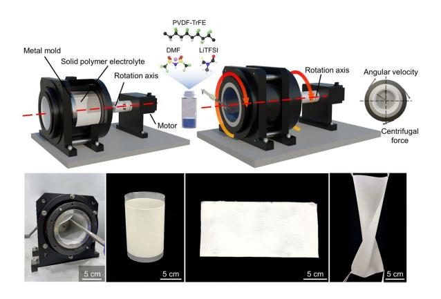
Depiction of the fabrication process for HCC-derived SPE, utilizing a custom apparatus accompanied by digital images of both the HCC and SPE films. Credit: *Energy Storage Materials* (2024). DOI: 10.1016/j.ensm.2024.103260
