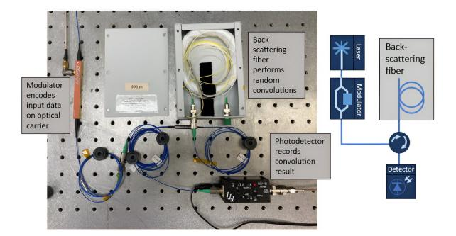
U.S. Naval Research Laboratory Optical Sciences Division's fiber optic computing experiment of encoded data on an optical carrier using the modulator, left, orange housing, and coupled into a 500 meter backscattering fiber, upperright, gray aluminum housing, which applies a series of random convolutions on the input data. The result of the convolutions is recorded on a high-speed photodetector seen in lower-right, black housing. Credit: U.S. Naval Research Laboratory
