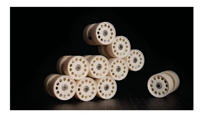
The Granulobot is composed of simple gear-like units with magnets. This design allows the individual units to move as a whole, much like a swarm of bees. Credit: Saintyves and Jaeger
