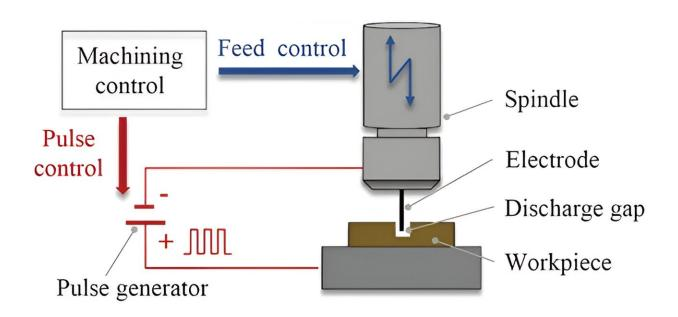
Schematic diagram of feed control and pulse control in micro-EDM. Credit: *Advances in Manufacturing* (2024). DOI: 10.1007/s40436-023-00471-z
