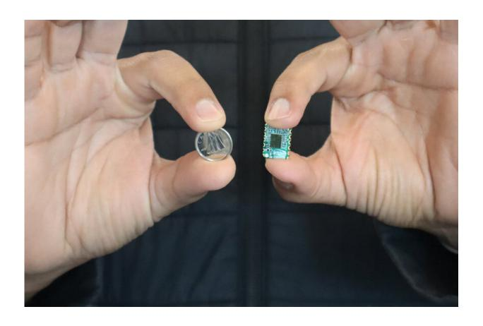
Radar sensor held up next to 10c coin to give size comparison. Credit: University of Waterloo
