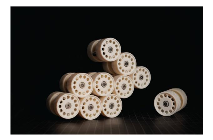
An aggregate of Granulobots, robotic units capable of self-assembling into cohesive, active and reconfigurable aggregates that exhibit tunable solid or liquid-
