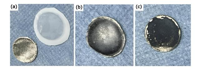
Optical images of lithium under three conditions: a) lithium foil with no FG coating (with electrolyte), b) FG pressed on Li foil without electrolyte, c) SEI formed after 2 days rest in FG@CM cell (with electrolyte). Credit: *Small* (2023). DOI: 10.1002/smll.202308344
