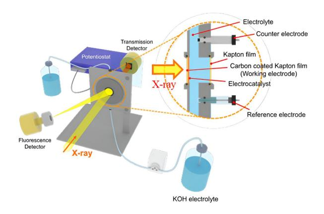
In-situ X-ray absorption spectroscopy instrumentation schematic. Credit: Korea Institute of Science and Technology
