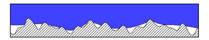
A schematic representation of a close up view of a liquid droplet (blue) on a solid substrate (striped) where surface roughness is apparent. The liquid-solid contact shows where air pockets (white) develop, introducing nucleation. Credit: Karim Alamé et al. 2020
