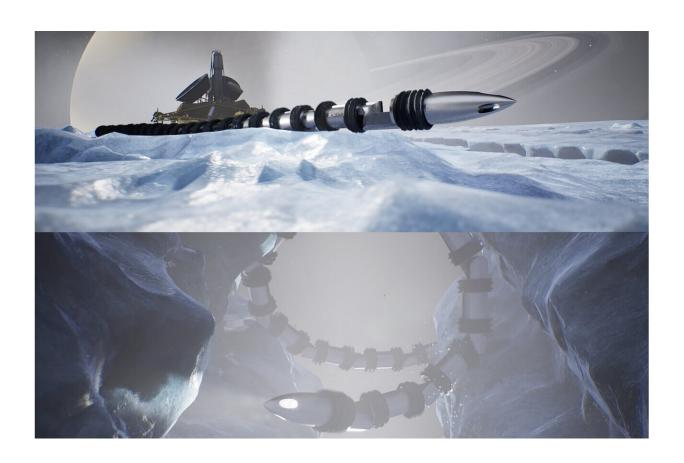
Artist renditions of the EELS concept. (Top) The system moving with the help of its active skin propulsion toward a vent after being deployed by a lander on Enceladus. (Bottom) The EELS platform climbing down a vent, resisting the upward fluid dynamic pressure by pushing out against the ice walls. Credit: NASA/JPL-CALTECH; from . *Science Robotics* (2024). DOI: 10.1126/scirobotics.adh8332
