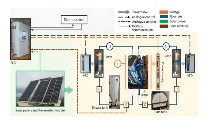
The system automatically adjusted the voltage and the rate at which salt water flowed through it dependent on variable levels of sunshine. By matching the workings of the machine to the available water power, the team could develop a system that cut down on expensive battery usage while not compromising on the amount of drinking water produced. Credit: *Nature Water* (2024). DOI: 10.1038/s44221-024-00213-w
