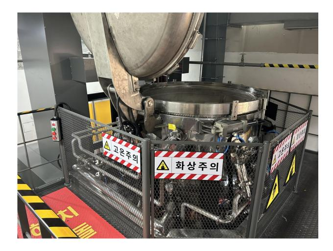
Medical waste treatment system capable of processing 100 kilograms of medical waste per hour, demonstrated at the Chungnam National University Hospital. Credit: Korea Institute of Machinery and Materials (KIMM)
