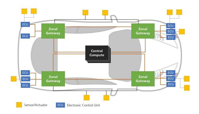
An automotive megatrend: A central supercomputer controls all car components and can be updated via a Wi-Fi connection. Credit: Fraunhofer-Gesellschaft
