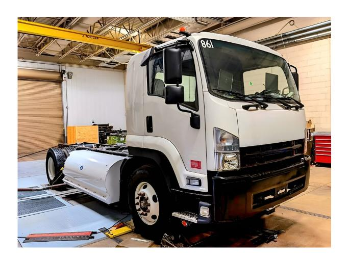
SwRI developed and demonstrated a state-of-the-art natural gas-fueled/hybrid powertrain for medium- and heavy-duty applications. The medium-duty natural gas hybrid demonstration truck reduced greenhouse gases by 25% relative to standard diesel-powered trucks. Credit: Southwest Research Institute
