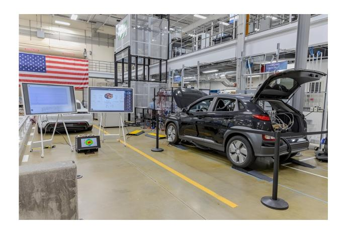
ORNL researchers achieved the highest wireless power transfer level for a light-duty passenger vehicle when the team demonstrated a 100-kW wireless power transfer to an EV using ORNL's patented polyphase electromagnetic coupling coil. Credit: Genevieve Martin/ORNL, U.S. Dept. of Energy
