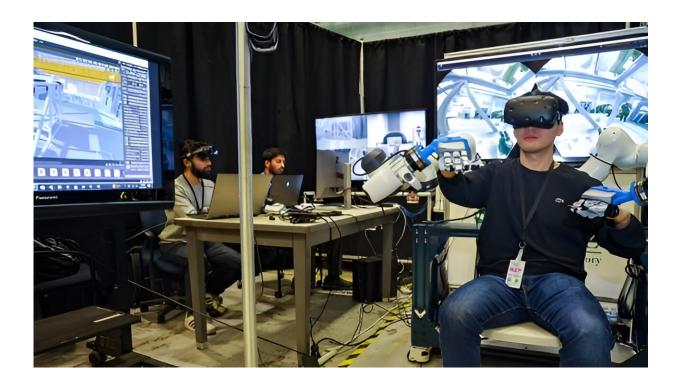
Designed by Argonne scientist Young Soo Park, a remote-controlled, dual-arm telerobotics system was successfully demonstrated at a long-closed radiochemical processing facility at ORNL. Operators equipped with a virtual reality headset and touch-sensitive haptic gloves can control the robots physically and virtually at the same time. Credit: Oak Ridge National Laboratory
