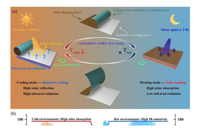
The newly developed Zero-Energy Switchable Radiative Cooler (ZESRC) automatically switches modes with temperature changes, cooling under high temperatures, and heating under low temperatures. Credit: *Journal of Photonics for Energy* (2024). DOI: 10.1117/1.JPE.14.028501
