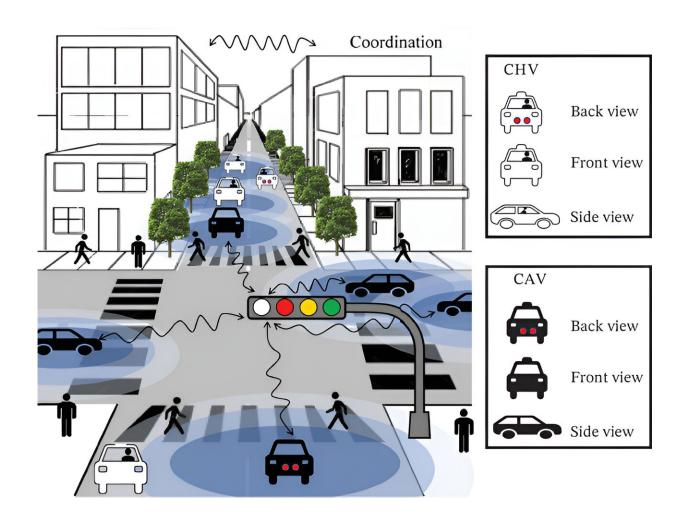
Schematics of an intersection with white phase, connected automated vehicles (CAVs), connected human-driven vehicles (CHVs), and pedestrians. Credit: *Computer-Aided Civil and Infrastructure Engineering* (2024). DOI: 10.1111/mice.13178
