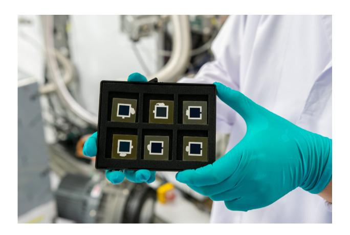
NUS researchers successfully integrated a new anion, cyanate, into a perovskite structure, which was a key breakthrough in fabricating new triple-junction perovskite/Si tandem solar cells. Credit: National University of Singapore
