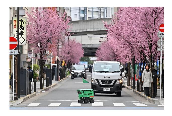
The robots calculate routes on their own, using sensors to avoid pedestrians and other obstacles.
