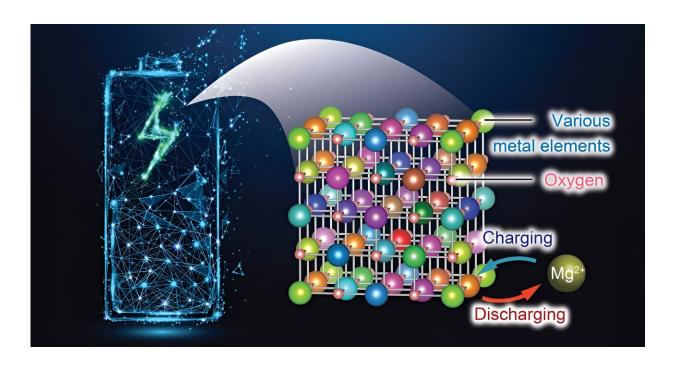
Schematics of the battery and present cathode material. The present material contains many metal elements as cations thanks to the effect of the high configurational entropy. Credit: Tohoku University
