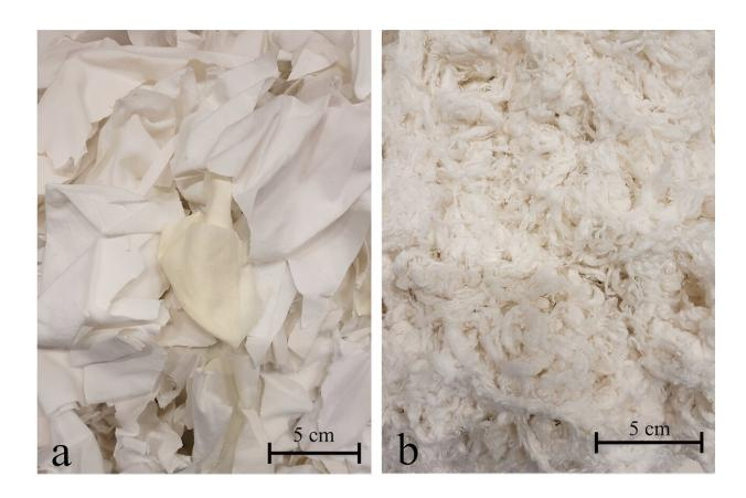
Cotton waste textiles before treatment (**a**) and the resulting dissolving pulp after low-consistency treatment with  $ZnCl_2\cdot 4H_2O$  (**b**). Credit: *Cellulose* (2023). DOI: 10.1007/s10570-023-05646-2
